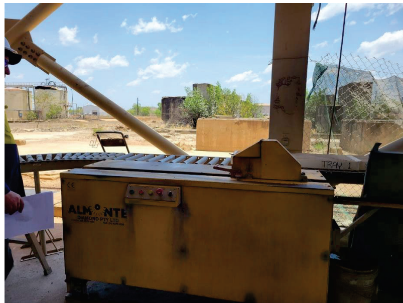
Figure 24 Saw Station for Core Cutting, Vista November 2024
